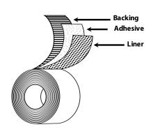
Backing:1.0 mil White Polyester FilmAdhesive:Heat Seal Rubber (1905)Liner:60lb semi-bleached kraft, silicone<br/>release treated on both sides
